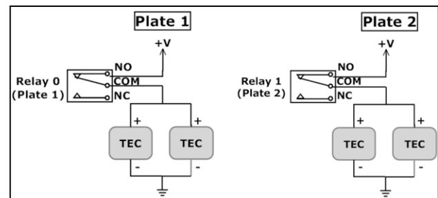
Figure 2. Schematic diagram of thermoelectric circuits. Under each plate, two thermoelectric modules (TECs), wired in parallel, are connected via the Normally Open (NO) contacts of a relay to a variable DC power source. When the computer closes the relay, current is supplied to the TECs and the device is cooled. Reversing the polarity at the power supply causes the TECs to warm upon activation rather than cool.
